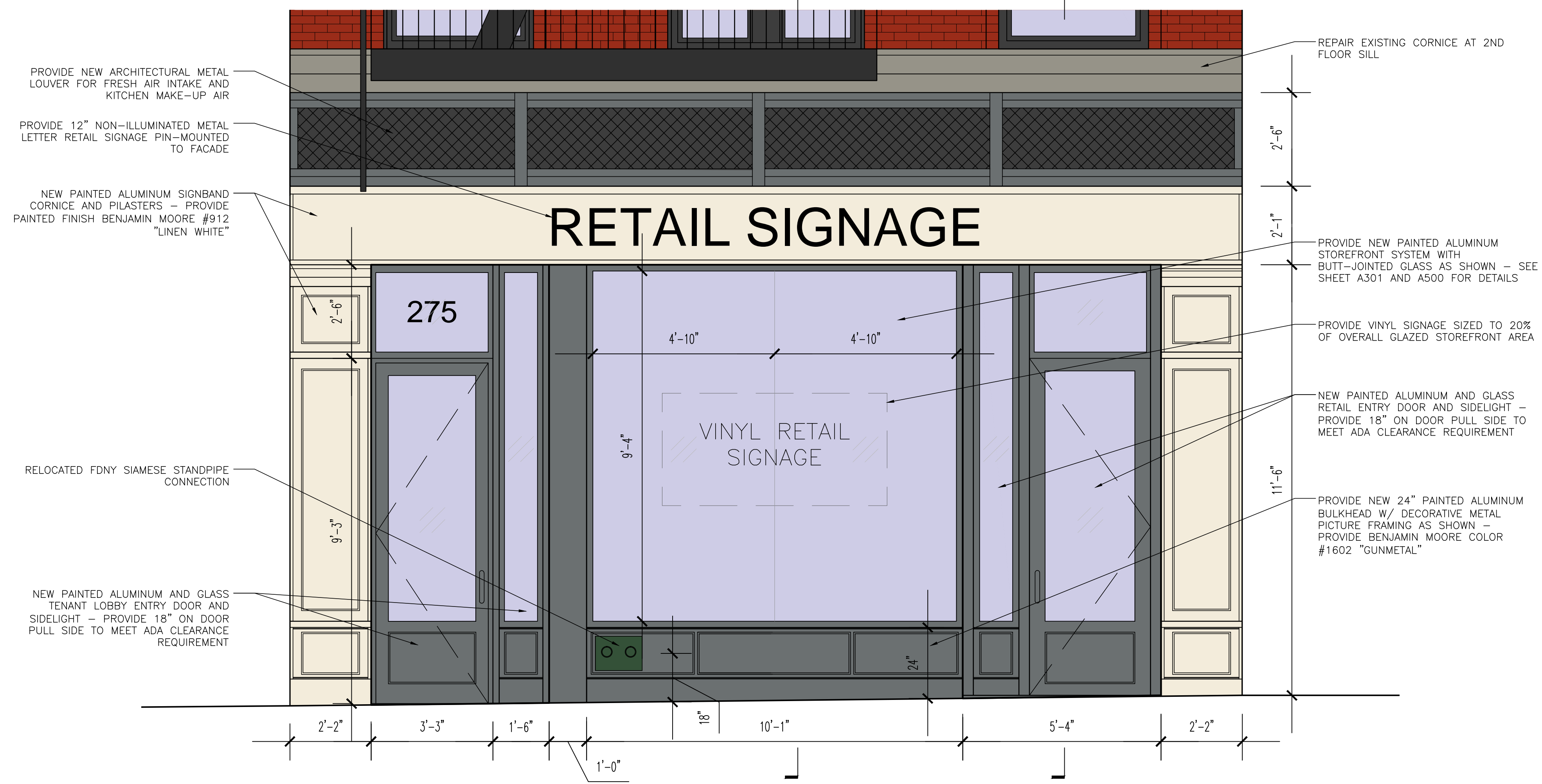
02 PROPOSED ENLARGED STOREFRONT ELEVATION 3/4" = 1'-0"
